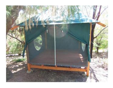
**Tea Room** with a Zippered Entrance wall open + tied back, and a Zippered Screen Entrance wall in its down position, with the bottom of the wall secured to the edge of the deck. (With "Moon Window" walls on the left and right, and a solid wall to the rear.)
