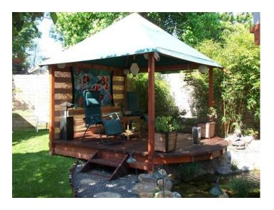
Another view on a **Tea Room** with a custom deck made out of high quality redwood floor boards and a cantilevered extension over a koi pond. In as similar manner, with the addition of custom floor joists, the standard 10' x 10' deck of the **Tea Room** can be extended on any one or more of its four sides.
