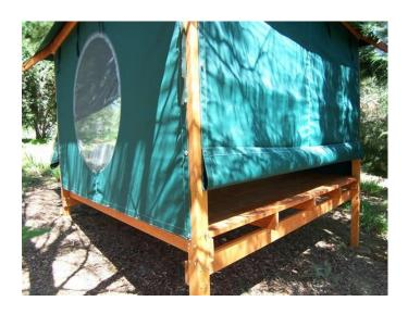
View on a **Tea Room** – the bottom edge of its Solid Wall has been turned up for added ventilation on a warm day. (With a "Moon Window" wall to the left, and two longer corner posts on the downhill side to accommodate the siting on sloped ground.)
